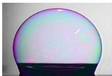
A soap bubble wetting an ultra hydrophobic surface
